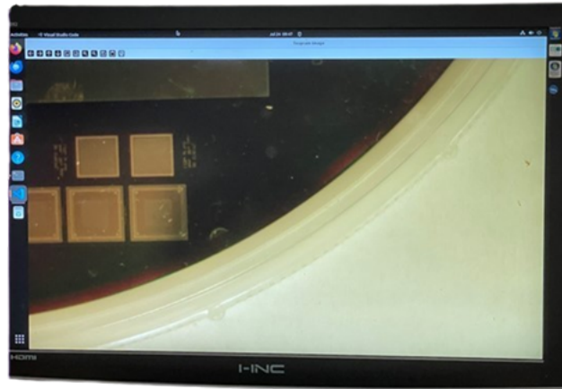
Figure 2a: A high-resolution image of a single section of the silicon wafer captured by the automated optical inspection system, showcasing the system's ability to produce detailed surface images for defect analysis.
