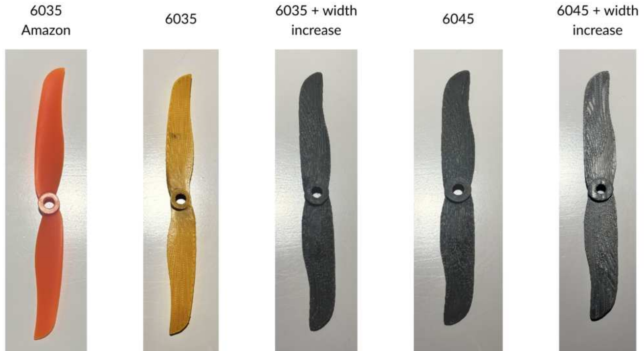
Figure 5: Blades after printing
