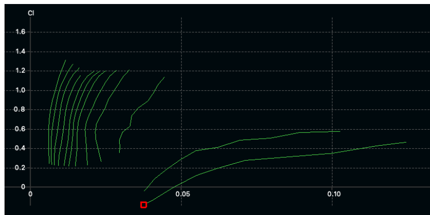
Figure 19: Airfoil 3.0 Cl vs Cd Plot; x-axis represents coefficient of drag, and y-axis represents coefficient of lift.
