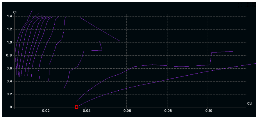
Figure 15: Airfoil 2.0 Cl vs Cd Plot; x-axis represents coefficient of drag, and y-axis represents coefficient of lift.
