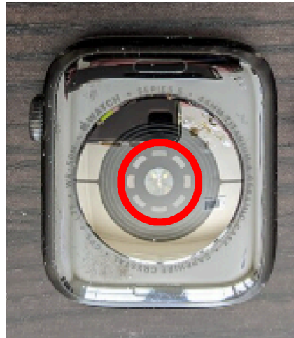
Figure 1 | Back of an Apple Watch and PPG sensor location. Photo by Mliu92 (CC BY-SA 3.0), cropped, with red circle added 2 .
